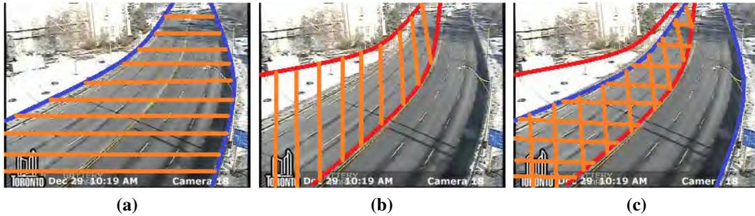
**Figure 4.3** Precision and recall calculation (a) human labelled ground truth road region by two boundaries (b) identified region by proposed approach, and (c) correctly identified region.
