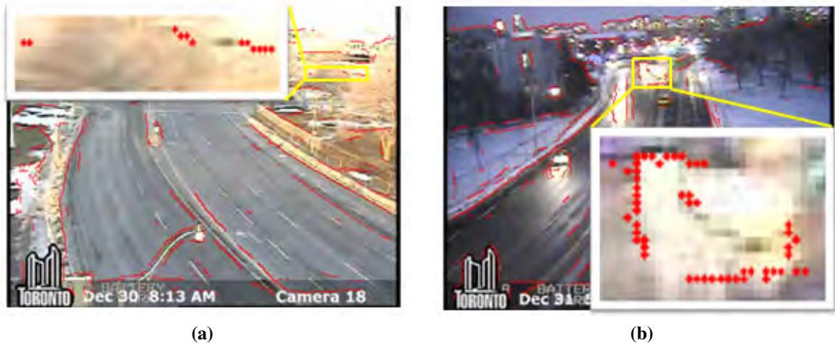
**Figure 3.5** Spurious edges generated in edge detection step for (a) blurriness of the traffic image, (b) vehicle headlight reflections.
