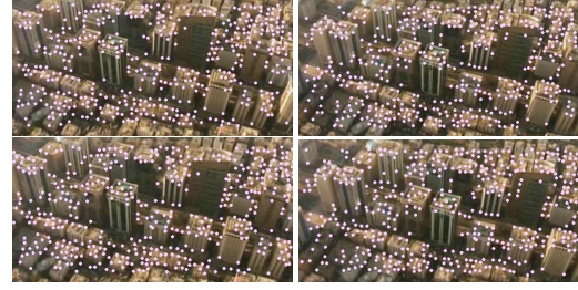
Figure 3. Intermediate (top row) and key (bottom row) mosaics generated from the Dubai sequence. The circle represent the SFM key points.
