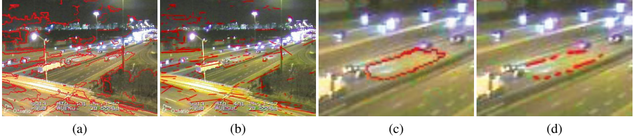
Fig 3: Polygon approximation using adaptive sampling. (a) Approximated polygons for superpixels in Figure 2e. (b) Same image in (a) but showing edges that are more than 10 pixels in length. (c) Showing a single superpixel from (a). (d) Edges more than 10 pixels for the superpixel in (c).
