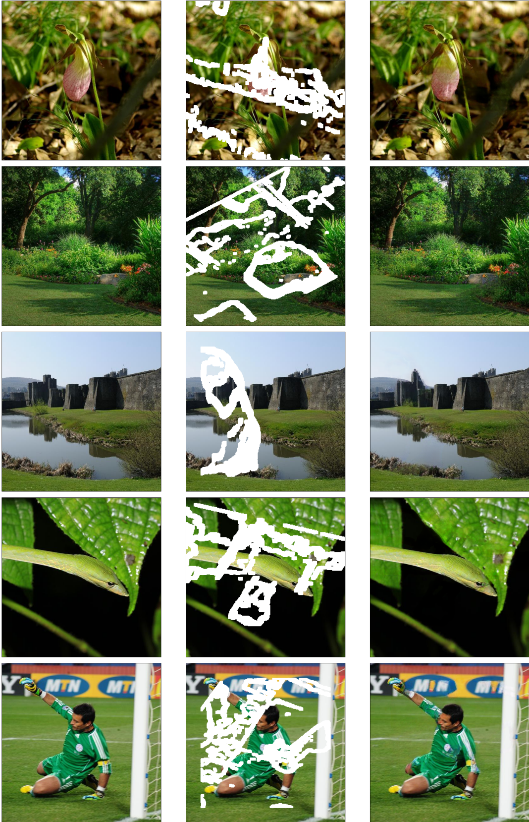
Figure 7: Sample of results with Places2 dataset ( 512 \times 512 ). Images are best viewed in color. From left to right: Original Image, Input Image, Generated Result.
